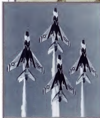
▼ Short-tail F-100A The first 70 production F-100As had shorter fins, which caused roll control problems.
